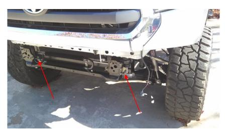
**Figure 3 - Factory Bumper Connection**
