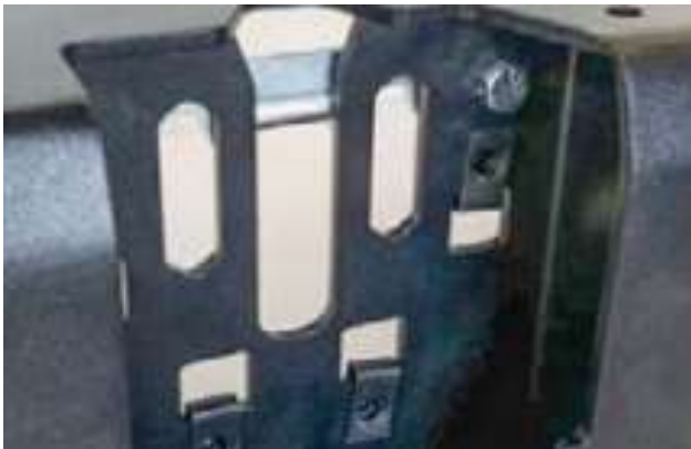
Welded Rod Plate should face inside the bumper and mounted in the upper most position.
