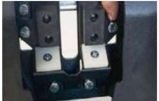
Adjust the Kickplate as needed for best arm contact and latch travel.
