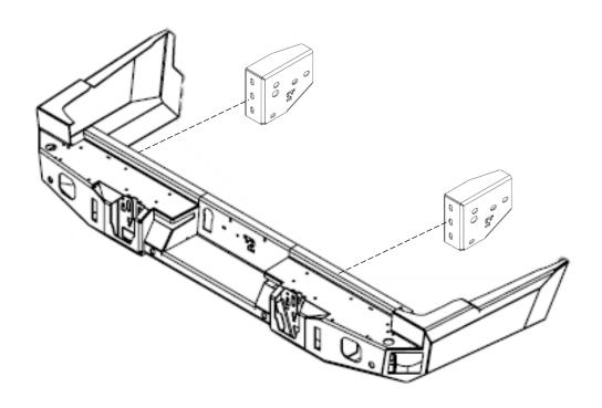
Pull the OEM plastic cap for both sides of the frame in the wheel well. First insert the single bolt retainer into the opening and place into location at the bottom bolt opening. Second in conjunction with step 11, insert the provided double nut retainer from the inside of the frame. Mount the side wing bracket once all nut retainers are in location.
