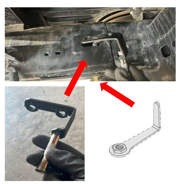
Use a socket extension as a handle to hold the nut retainer in place.
