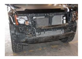
Remove frame piece as shown to right with the few remaining bolts that are holding it in place.
