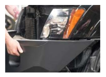
Carefully insert the provided frame bolts/washers into the frame holes with the bumper lined up. Secure with provided washers/ nuts. If you're happy with bumper alignment, go ahead and tighten down all nuts and bolts on the frame brackets and the bumper.
