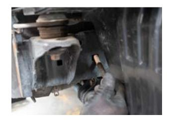
Slide the included small frame bracket next to the body frame as shown on drivers side. Bolt is pushed through frame and bracket as shown in previous photo. Tighten with included washer and nut.
