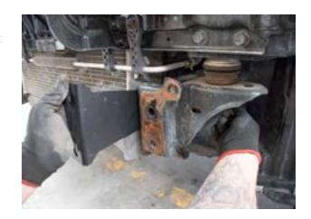
We recommend hand tightening the small frame bracket with the two bolts and included washers and nuts to loosely attach to the larger frame bracket as shown in photo.
