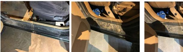
I. REMOVE PHILLIPS SCREWS AND REMOVE FRONT AND REAR ROCKER PLASTIC PANELS.
