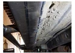
5. FULLY FINISH WELD. WELD IN 6" SECTIONS MOVING AROUND.
