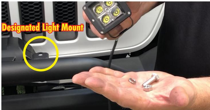
3. Utilize the provided hardware to fasten the light onto the two designated light points on the Scorpion bumper.
